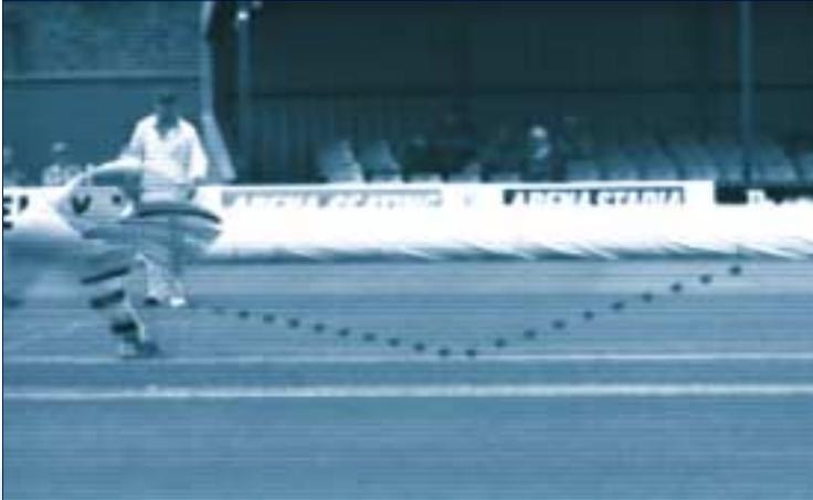
*Superimposed high speed video images of the cricket ball trajectory (blurred image of batsman to the left).*
