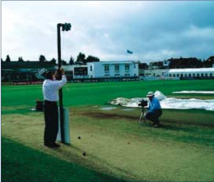
*The three metre ball drop test.*
